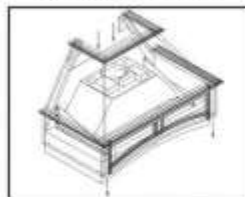
Step 5: Slip the wood range hood on top of the mounting plate
