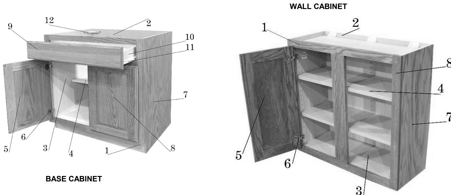
1. 3/4" HARDWOOD FACE FRAMES WITH GLUED AND POCKET SCREWED JOINTS.
